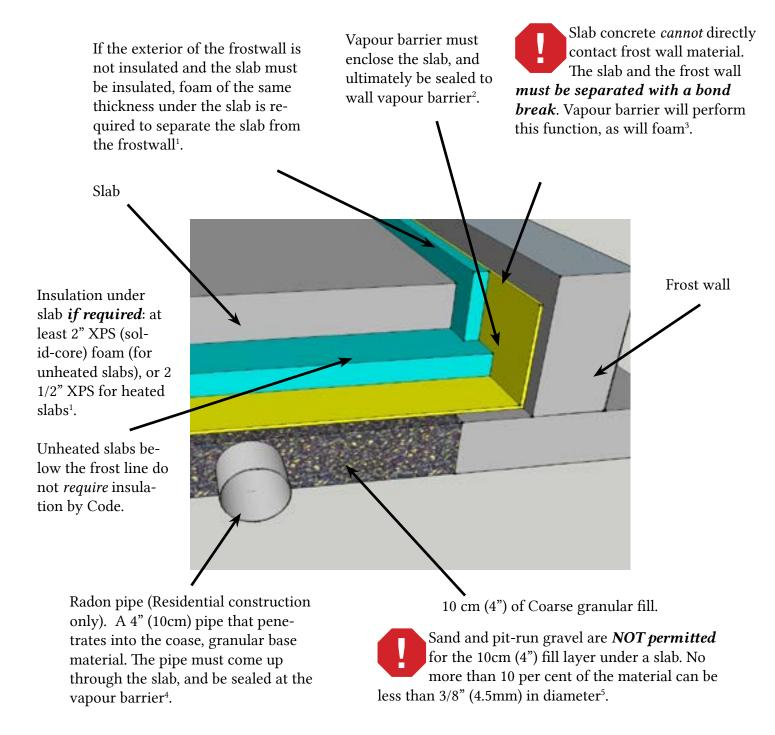
Code (2015) references: [1] Table 9.36.2.8-A or 9.36.2.8-B. [2] 9.25.3.3(3) XPS foam ok as air barrier, as long as vapour barrier sealed to it or overlapped. [3] 9.16.4.4 [4] 9.13.4.3 [5] 9.16.2.1
